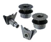
The adjustment tool supplied as standard equipment, used to transfer the distances between the holes of the board and for quick and accurate setting of the CUTBEND
